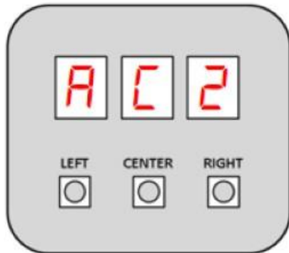
Air Conditioner – High Stage
